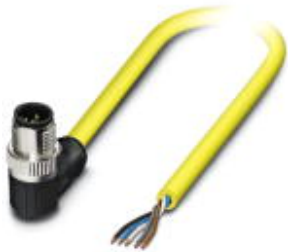
Sensor/Actuator cable, 5-position, PVC, yellow, Plug angled M12 SPEEDCON, A-coded, on free cable end, Cable length: 2 m
